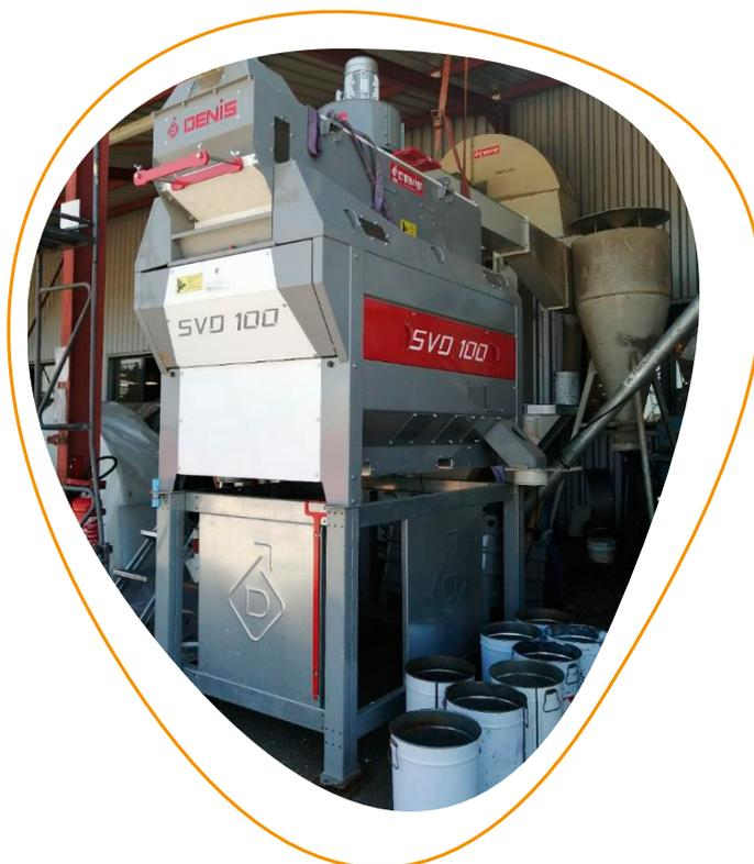
**Fig. 4.** Vibrating cleaner SVD100 from Etablissements Denis used to demonstrate the feasibility of the separation of species mixture and the resulting economic benefit (Picture from Patrick Bourachot)
